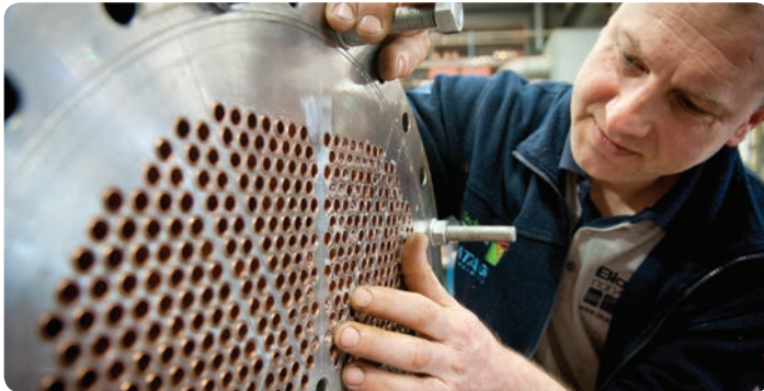
Reparatie van warmtewisselaars Retubing heatexchangers
